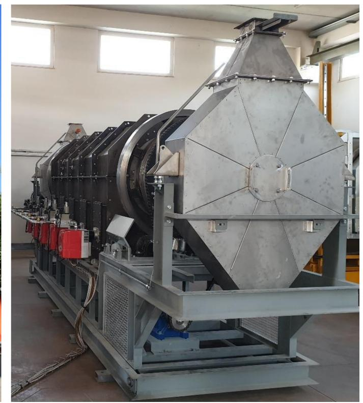
Lead Oxide Regeneration Unit – Pilot Plant
