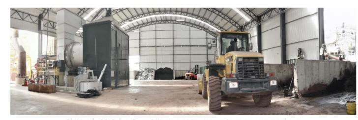
Pb Metals 2012: L to R - refining crucible - rotary furnace - storage bays
